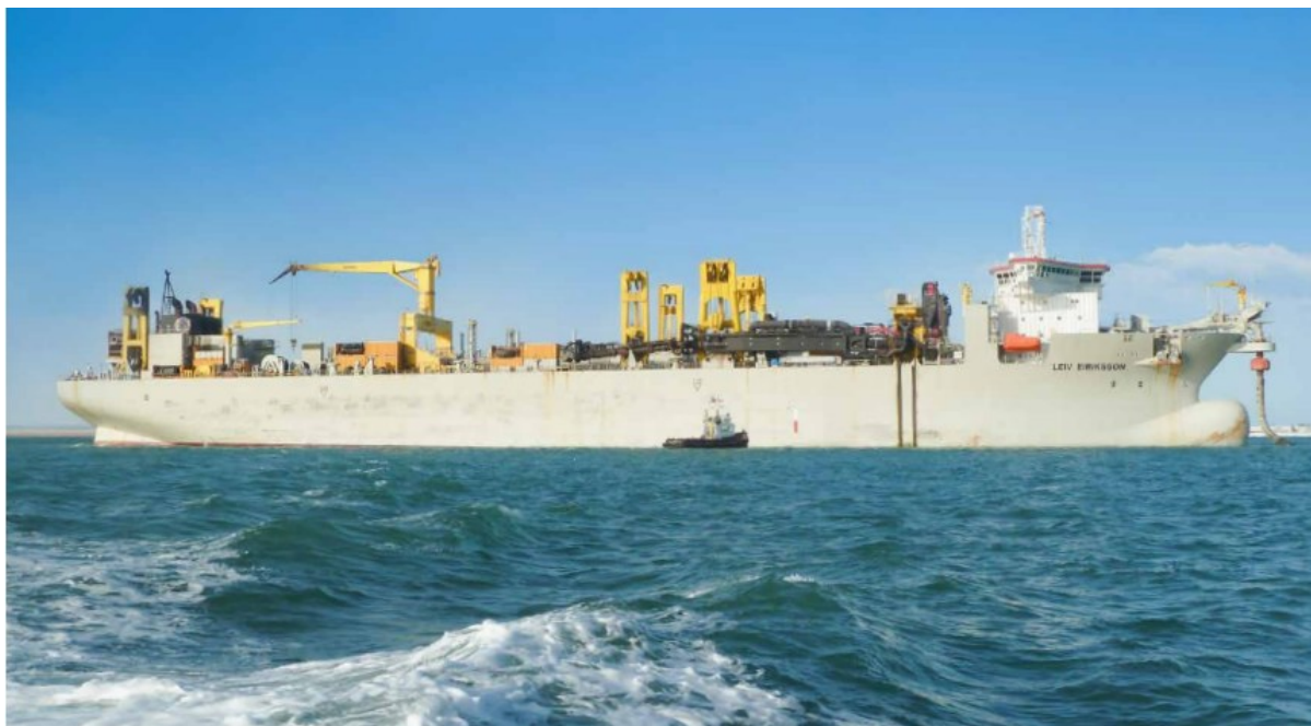
Figure 3.7 Example of a trailing suction hopper dredger (source: https://www.jandenul.com/sites/default/files/2020-05/Leiv%20Eiriksson%20%28EN%29.pdf )
