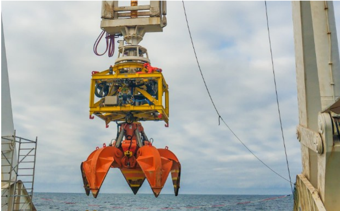
Figure 3.10 AssoGrapple II – a multi-purpose tool designed for seabed intervention (source:
